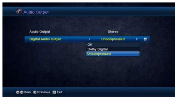
The digital receiver can output two types of digital audio signals via S/PDIF connector. One is an encoded signal
